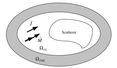
Figure 4. A conformal PML configuration.
