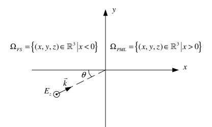
Figure 2. A  $TM_z$  plane wave incident to a PML half-space.
