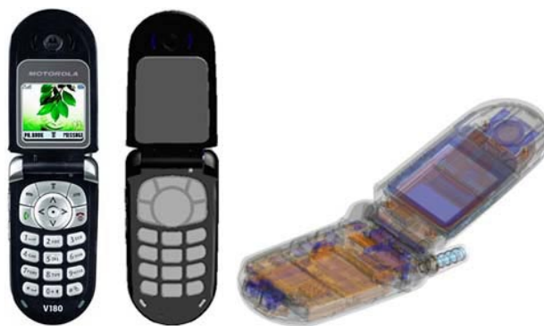
Figure 1. Multiband phone used in this study: photograph of the actual phone (left) and the CAD derived model.
