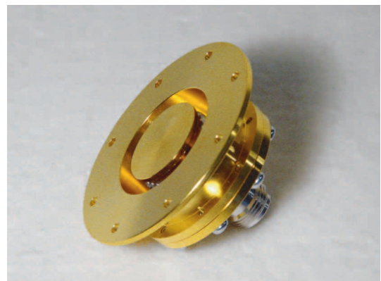
Figure 7. Existing IEC 61000-4-2 Ed1 "pelligrini target" approx. 1 Ghz.
