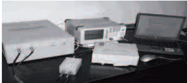
Figure 5. Photograph of the conductive electromagnetic interference noise measurement equipment.
