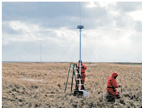
Figure 3. Picture of 5 MHz long-range SeaSonde. The receive antenna is shown in the foreground on the right. The transmit antenna is shown in the background on the left. Technicians installing the radar are shown for scale.
