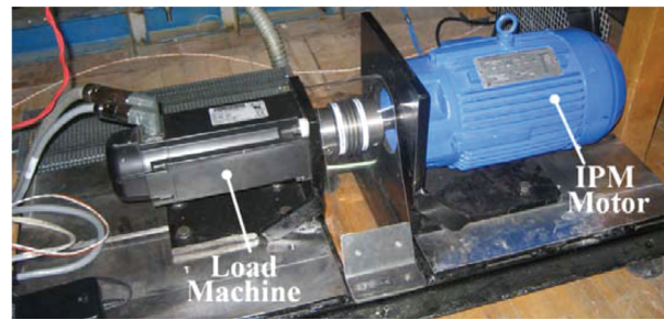
Figure 13. IPM motor experimental setup.
