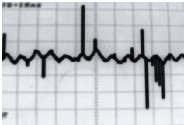
Figure 10c. The magnetic flux density traced with the z-sensor (CH 1 = \sim 0.5 V, TB = 10 ms, 1 mV \equiv 3/2 mG).
