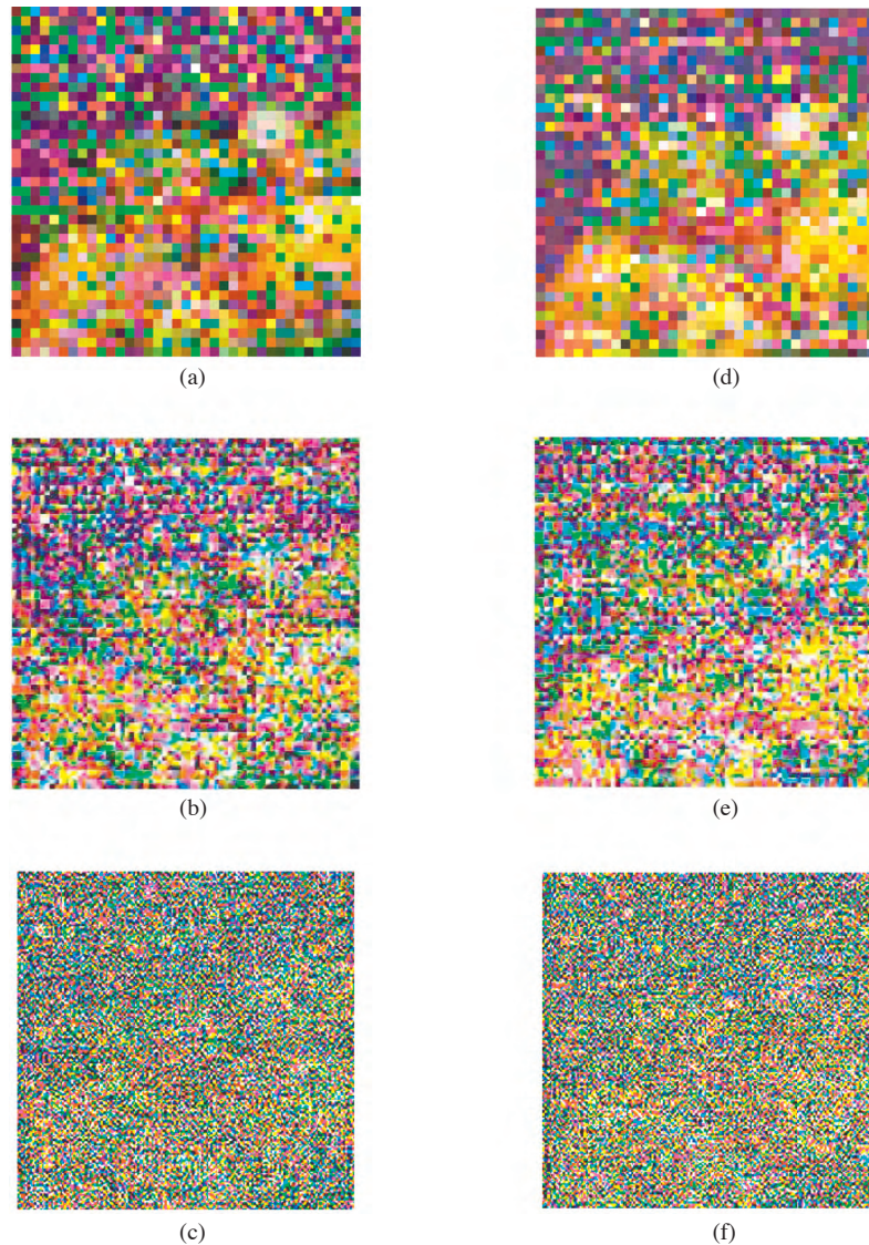
Figure 5. Reconstructed image for SNR = 2dB for a Rayleigh channel. (a) Total 96.875% compression (with 87.5% JPEG and 75% bit plane), (b) Total 93.75% compression (with 75% JPEG and 75% bit plane), (c) Total 87.5% compression (with 50% JPEG and 75% bit plane), (d) Total 93.75% compression (with 87.5% JPEG and 50% bit plane), (e) Total 87.5% compression (with 75% JPEG and 50% bit plane), (f) Total 75% compression (with 50% JPEG and 50% bit plane).
