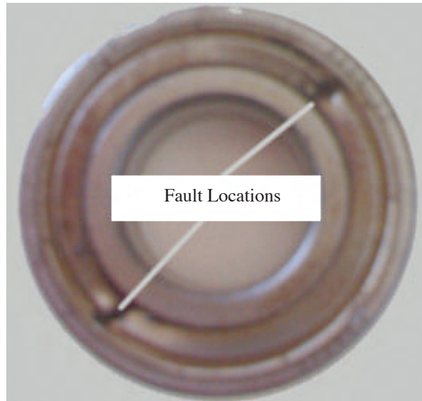
Figure 8. Artificially created bearing fault.
