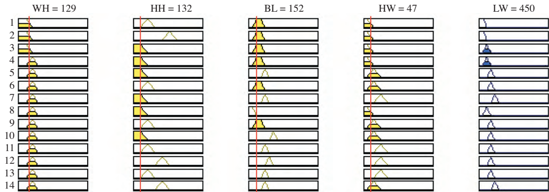
Figure 6. An example for LW prediction interactive interface generated by software with centroid defuzzification.
