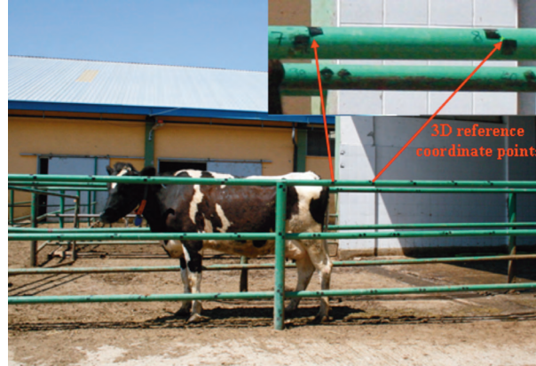
Figure 3. 3D reference coordinate points fixed on the area created for the process of taking photos from sidelong perspectives.
