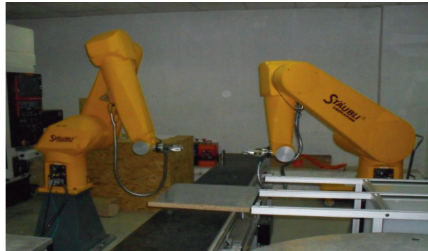
Figure 9. Staubli RX 160 and RX 160L serial robot arms.
