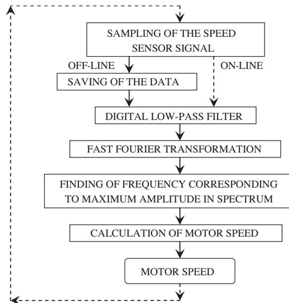
Figure 2. The block schema of the proposed algorithm.
