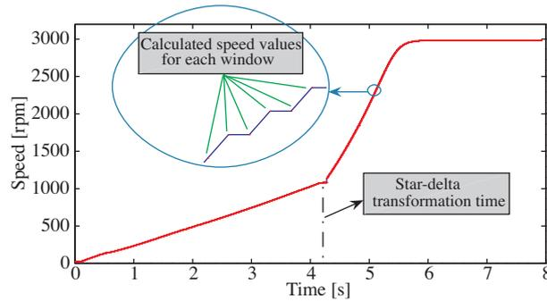
**Figure 4.** Experimental rotor speed-time curve during start-up using the FFT.
