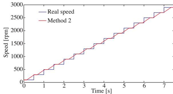
**Figure 6.** The obtained speed curve according to Method 2.
