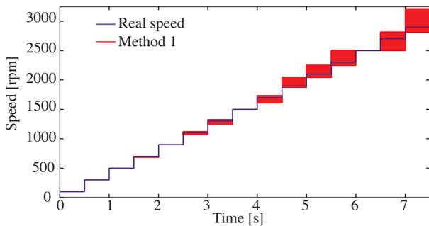
**Figure 5.** The obtained speed curve according to Method 1.
