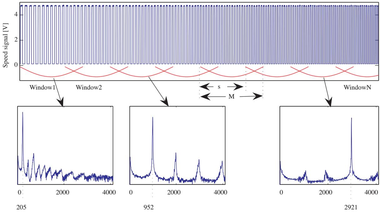
**Figure 3.** Speed sensor signal and evaluation of the maximum frequency values by the FFT.
