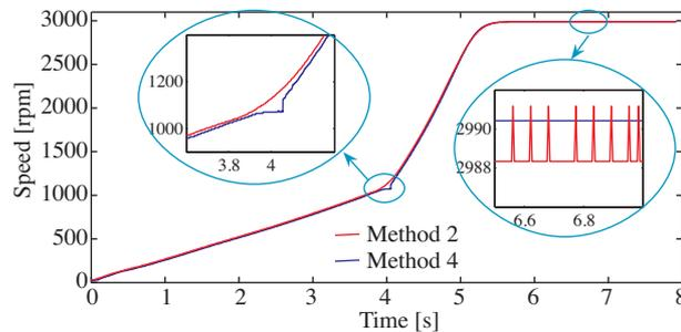
**Figure 14.** Comparison of the speed-time curves using Method 2 (with hopping) and Method 4.
