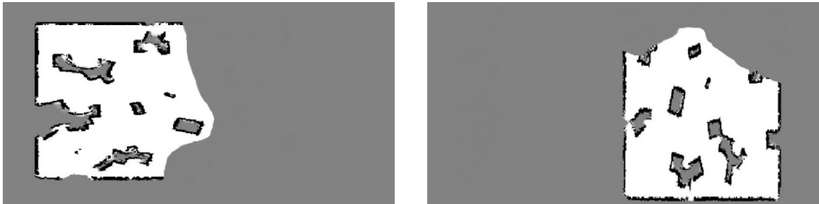
Figure 6. Partial environment occupancy grid map of the robots: a) first robot and b) second robot.
