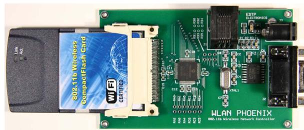
**Figure 2.** AirDrop-P card [1]. When the LWP protocol is loaded into the flash program memory, the overall embedded system is called the Airdrop-LWP.
