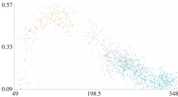
Figure 8. Relation between actual friction coefficient values and heat values. X-axis: heat, Y-axis: friction coefficient.
