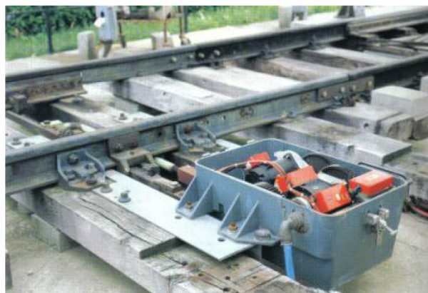
Figure 2. Currently used motorization for the shunting system.
