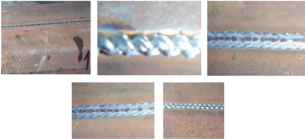
Figure 7. Different welding patterns that could be obtained by changing the welding parameters in the algorithm.
