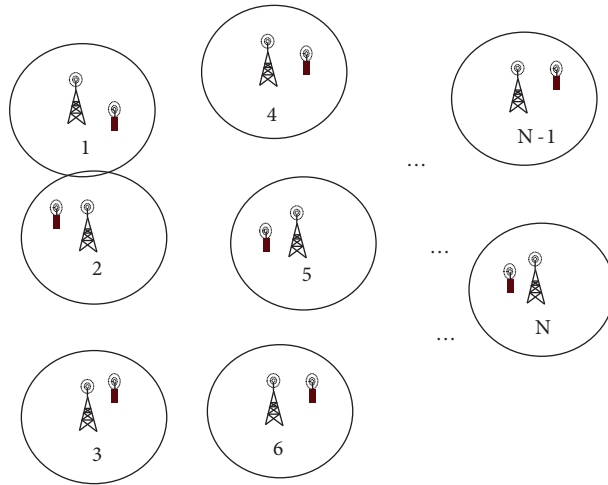
Figure 1. A wireless network with N BSs and N co-channel MSs.
