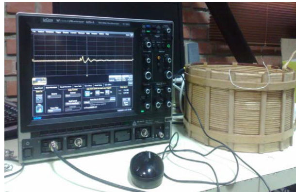
Figure 11. A view of the test done on a 20-kV transformer winding in a lab setting.
