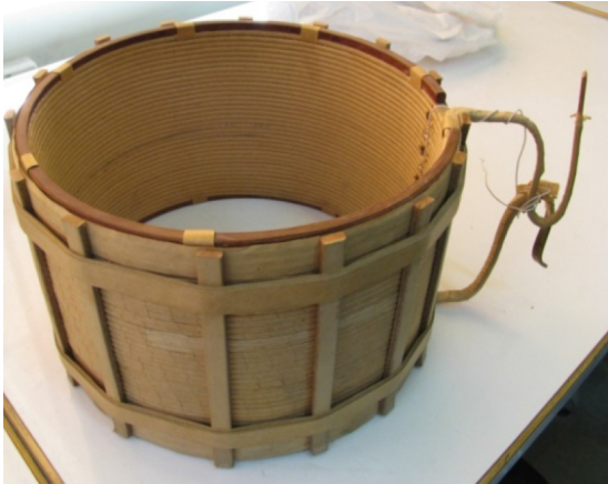
Figure 3. The 20-kV transformer winding.
