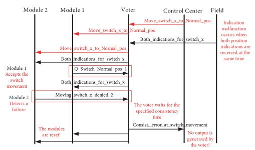
Figure 15. An example sequence diagram for a type 2 problem.
