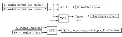
Figure 11. Prevention of the switch movement when its block is occupied.
