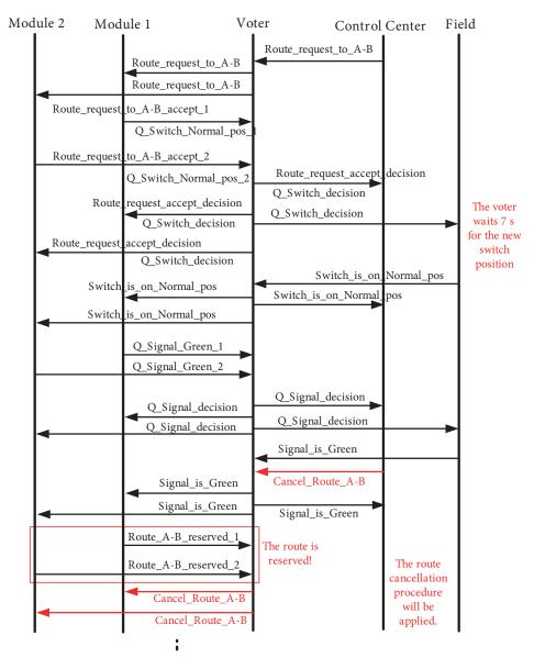
Figure 14. The sequence diagram of a possible solution for a type 1 problem.
