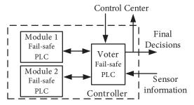
Figure 3. The structure of the controller (the voter and the modules).
