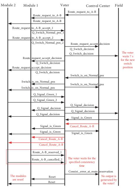
Figure 12. An example sequence diagram for a type 1 problem.
