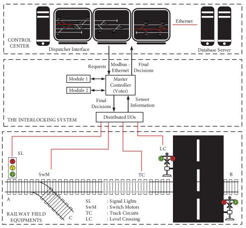
Figure 7. The general framework of a railway signaling system.
