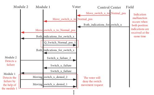
Figure 17. A sequence diagram of a possible solution for a type 2 problem.
