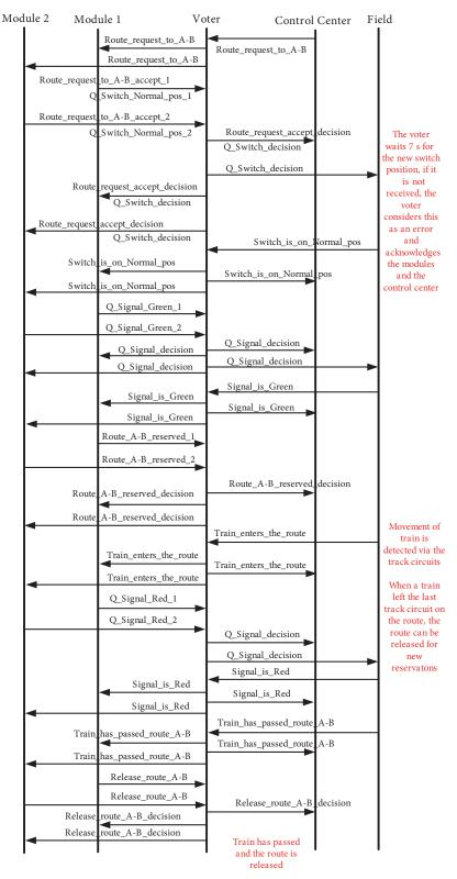
Figure 8. The sequence diagram for reservation of route A–B.
