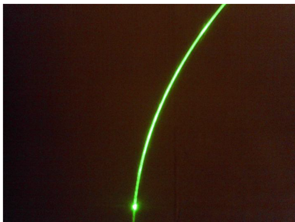
Figure 5. Bending of green laser light towards the right (dimensions of the photo: 500 × 700 mm).
