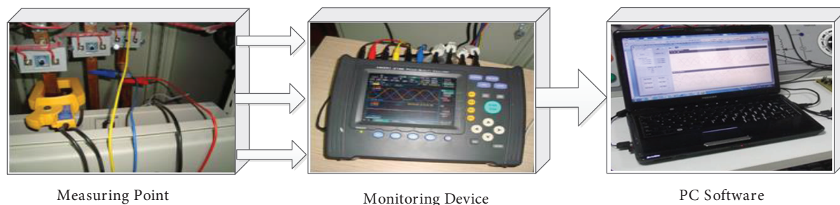
Figure 1. Harmonic monitoring system.
