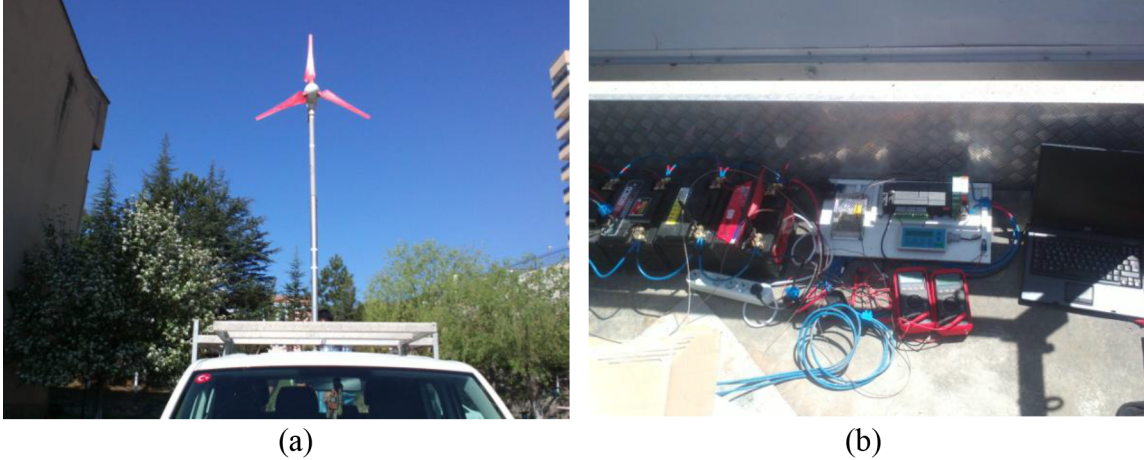
Figure 1. (a) The truck test; (b) the setup of the measuring system of the MWT.
