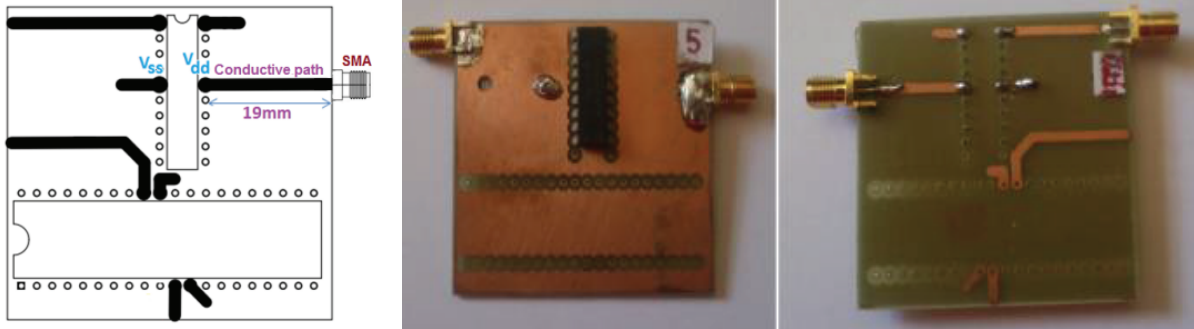
Figure 2. Designed and measured test circuit.
