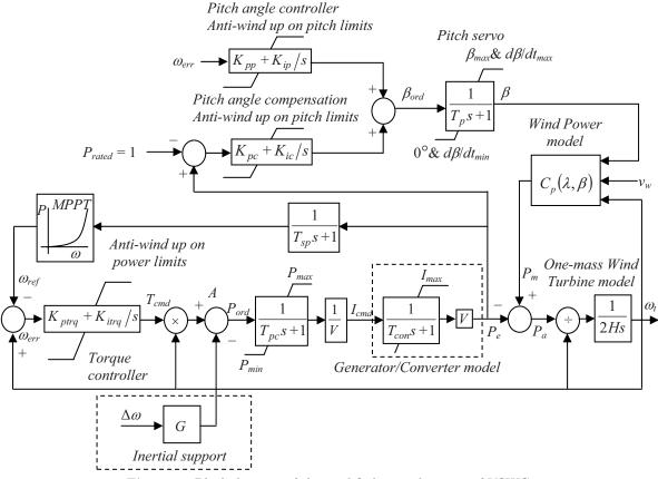
Figure 3. Block diagram of the modified control system of VSWG.
