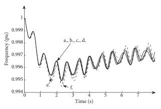
Figure 9. Frequency deviation after an active power disturbance of 30 MW: with inertial support as in Figure 3 (solid line for wind speed: a. 11.5 m/s, b. 8 m/s, and c. 3.5 m/s), and with inertial support as in Figure 2 (dash dotted line for wind speed: d. 11.5 m/s, e. 8 m/s, and f. 5 m/s).
