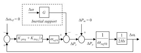
Figure 4. Linear control structure of the modified VSWG control algorithm with added inertial frequency support.
