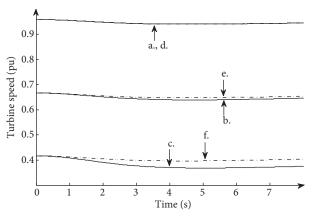
**Figure 11.** The VSWG speed after an active power disturbance of 30 MW: with inertial support as in Figure 3 (solid line for wind speed: a. 11.5 m/s, b. 8 m/s, and c. 5 m/s), and with inertial support as in Figure 2 (dash dotted line for wind speed: d. 11.5 m/s, e. 8 m/s, and f. 5 m/s).
