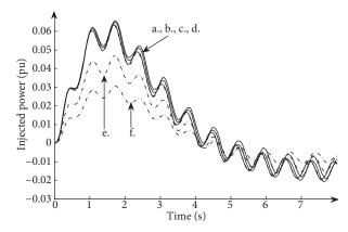
Figure 10. Injected power after an active power disturbance of 30 MW: with inertial support as in Figure 3 (solid line for wind speed: a. 11.5 m/s, b. 8 m/s, and c. 3.5 m/s), and with inertial support as in Figure 2 (dash dotted line for wind speed: d. 11.5 m/s, e. 8 m/s, and f. 5 m/s).
