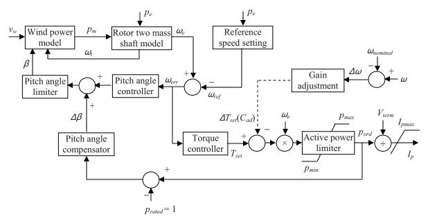
Figure 2. Schematic diagram showing active power and pitch angle controllers of DFIG (adopted from [14]).
