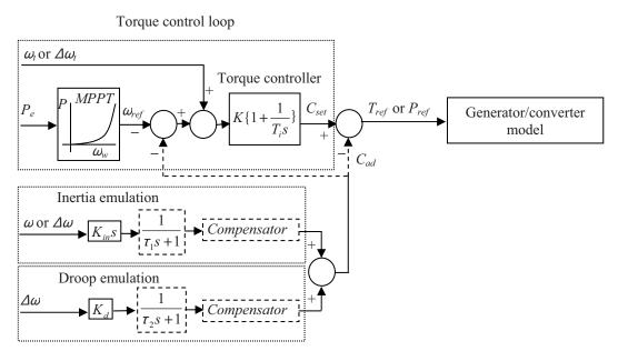
Figure 1. Control loops for wind unit active power control.
