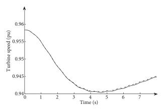
Figure 8. VSWG speed after an active power disturbance of 30 MW (wind speed 11.5 m/s): with inertial support as in Figure 3 (solid line) and Figure 2 (dash dotted line).
