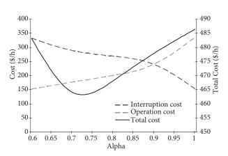
Figure 7. Interruption, operation, and total cost of redispatch with different values of  $\alpha_l$  in the nonlinear method.
