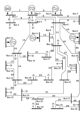
Figure 2. Single-line diagram of the IEEE 30-bus test system.
