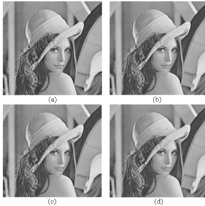
Figure 10. Lena-embedding results: (a) original, (b) 48.79 dB embedded with 0.27 bpp with [T_n, T_p] = [-1,0] , (c) 38.41 dB embedded with 0.86 bpp with [T_n, T_p] = [-5,5] , (d) 36.23 dB embedded with 0.97 bpp with [T_n, T_p] = [-12,12] .
