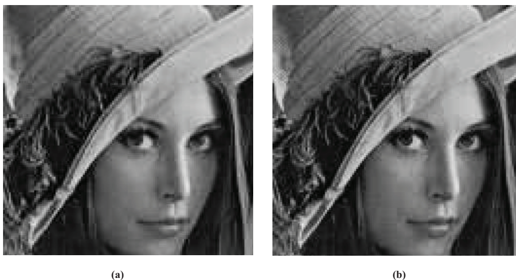
Figure 13. Reconstructed image by (a) JPEG quantization table and (b) KBGA quantization table.
