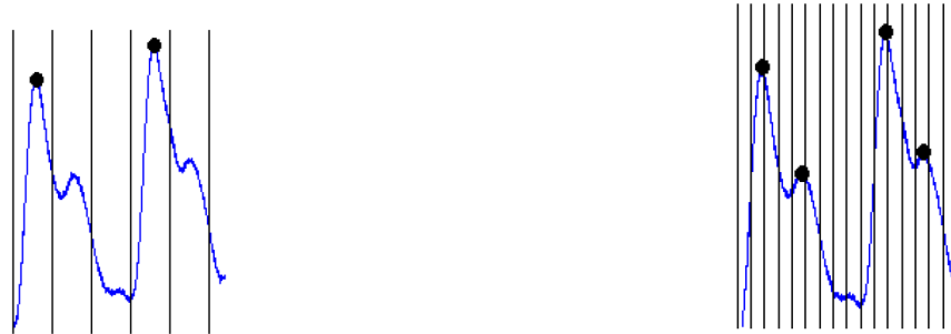
a) Two peaks detected in PPG signals by optimum segment points (correct estimation). b) Four peaks detected in PPG signals by big segment points (wrong estimation).
