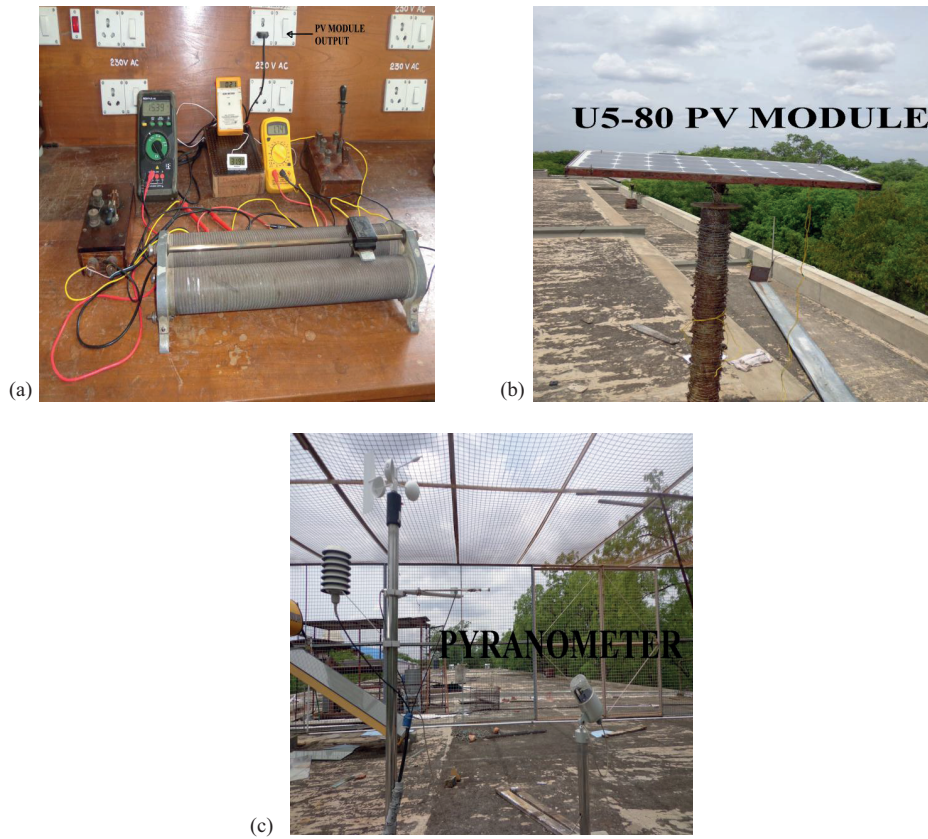
Figure 6. (a) Experimental setup of U5-80 PV module, (b) solar panel, (c) pyranometer.
