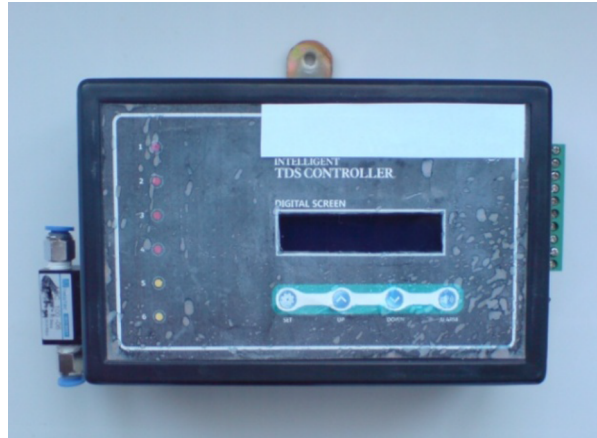
Figure 27. Schematic view of the TDS measurement and control system designed and manufactured in this work.
