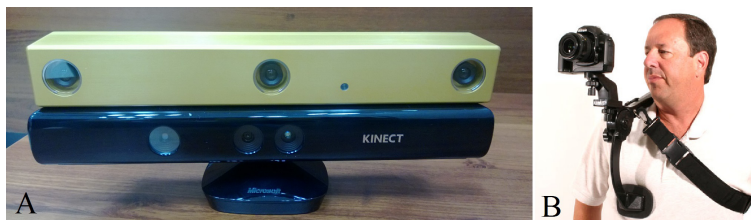
Figure 6. The system components. A) Kinect plus Bumblebee XB3 stereo rig used in the system. B) Padded shoulder image stabilizer for image acquisition. Brand name: RPS. These components along with a notebook PC allow for fine 3D reconstruction of outdoor scenes in rough terrains.
