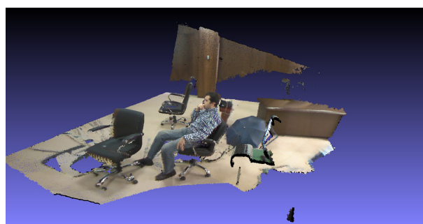
Figure 4. KinectFusion algorithm's limit for the reconstruction size is demonstrated. In the image there is a sharp slanted edge on the left side, which is the border of the allowable volume for reconstruction. Even though the Kinect sensor gathers data to the left of this border, it cannot be included in the 3D model due to memory limitations.
