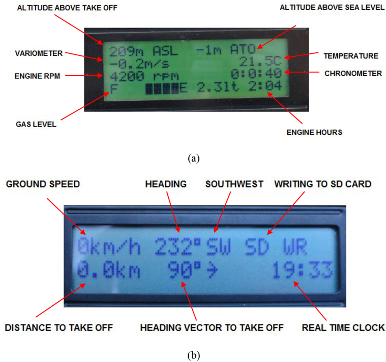
Figure 11. Engine (a) and GPS (b) LCDs during flight mode.
