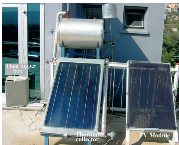
Figure 16. Thermal collector and solar module under test.
