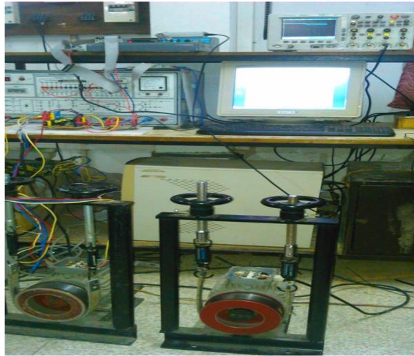
Figure 5. Experimental setup of parallel connected induction motor drive controlled by DSP TMS320F2812.
