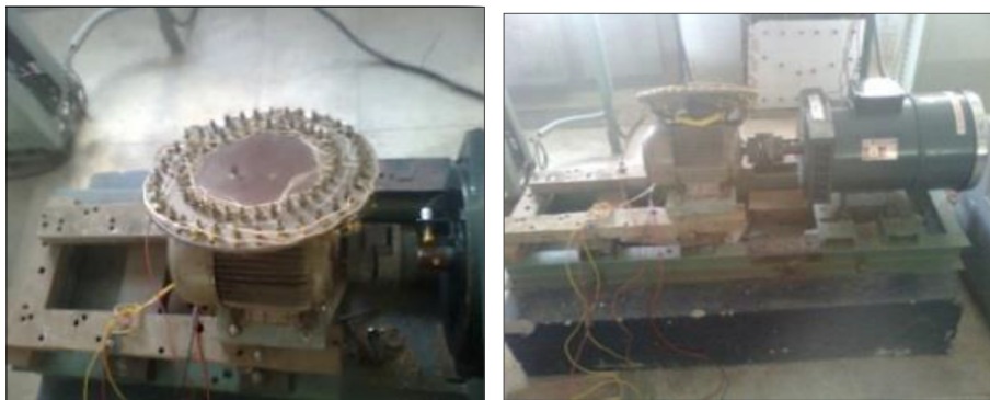
Figure 3. Laboratory set-up with stator winding arrangement.
