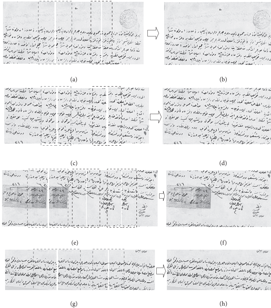
Figure 5. A sample historical document, namely a kushan, to illustrate the horizontal scanning phase of the video mosaicing algorithm with intermediate steps. (a) Three frames of the 1st row and two overlapping regions with dashed lines, (b) rowwise mosaic image of the 1st row. (c) Three frames of the 2nd row and two overlapping regions with dashed lines, (d) rowwise mosaic image of the 2nd row. (e) Four frames of the 3rd row and three overlapping regions with dashed lines, (f) rowwise mosaic image of the 3rd row. (g) Three frames of the 4th row and two overlapping regions with dashed lines, (h) rowwise mosaic image of the 4th row. (historical document source: http://www.telaviv-fever.com/index.php/2009/05/a-kushan-an-ottoman-land-deed/ )
