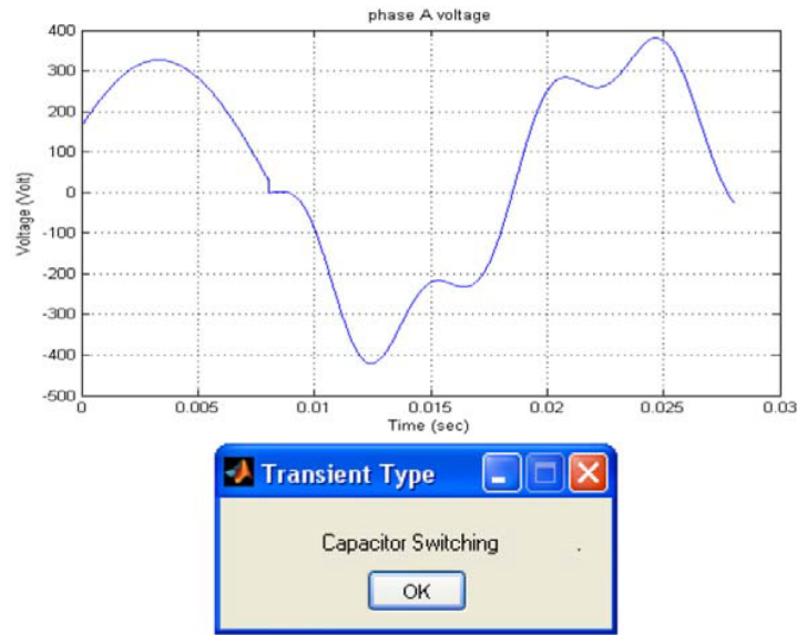
Figure 11. Voltage diagram and the output associated with simultaneous switching of three capacitors.
