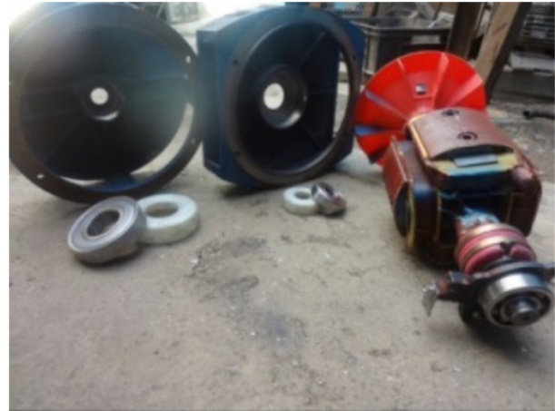
Figure 8. Insulation of synchronous generator bearings.
