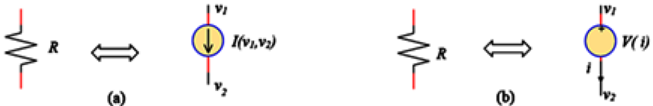
Figure 3. The equivalent of resistor: a) dependent current source, b) dependent voltage source.
