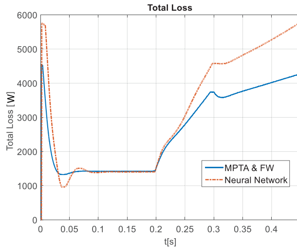
Figure 17. Comparison of total power loss variations between neural network and MTPA and FW control methods.
