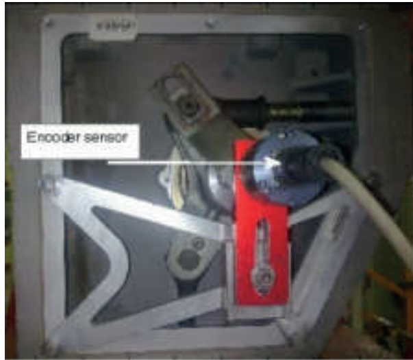
Figure 7. Real travel curve measurement system [20].
