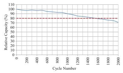
Figure 2. Relative capacity over cycle number graphic for the battery.
