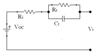
Figure 1. Electrical equivalent circuit battery model.
