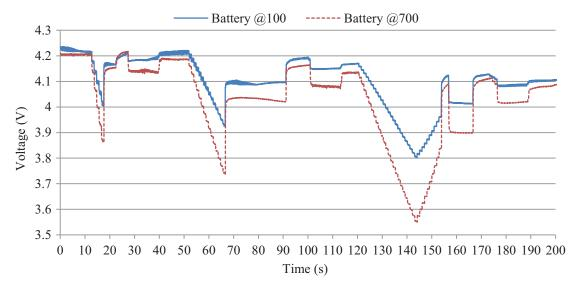
Figure 4. Reaction of two different aged batteries to the same driving cycle.
