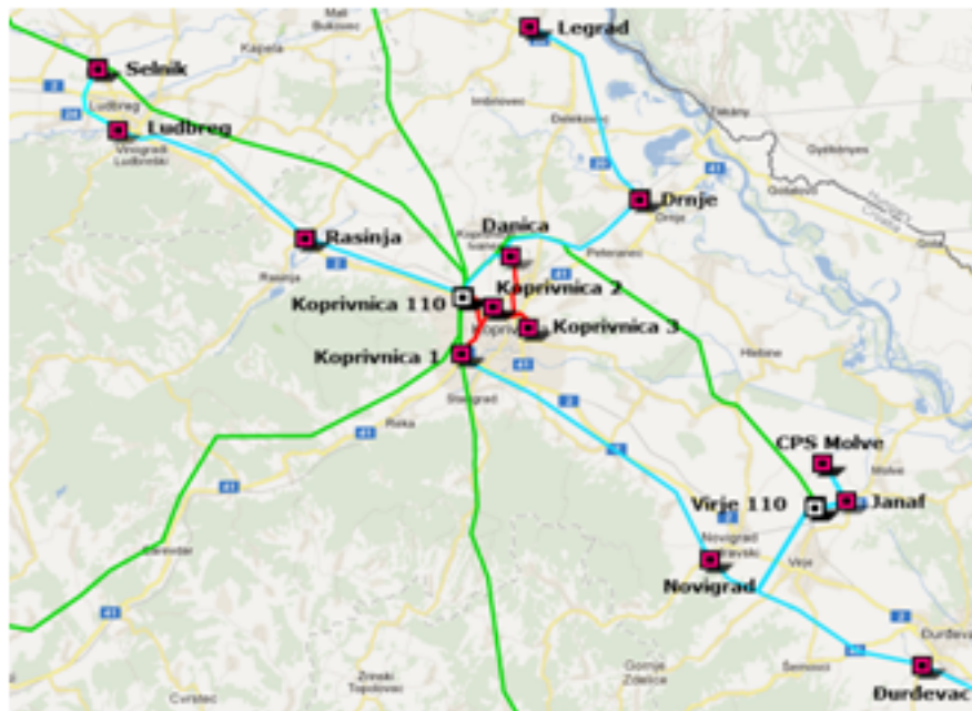
Figure 3. Geographical representation of 110 and 35 kV network of a Croatian DCA (green – 110 kV lines; blue – 35 kV lines; red – 35 kV cables).
