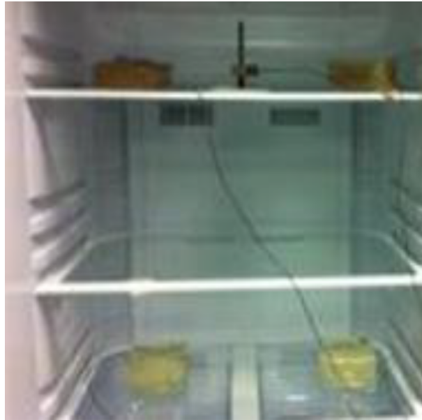
Figure 13. Standard test loads and open air thermocouple.
