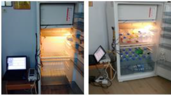
Figure 11. Refrigerator test condition a) no-load, b) with load.
