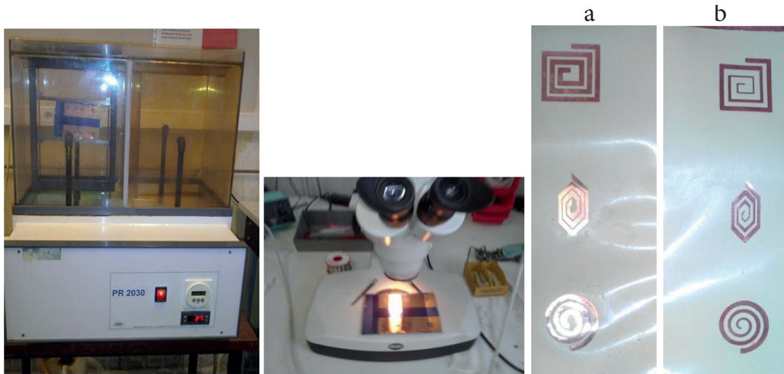
Figure 6. System of chemical etching (left) and topologies realized (right): (a) standards, (b) tapered.
