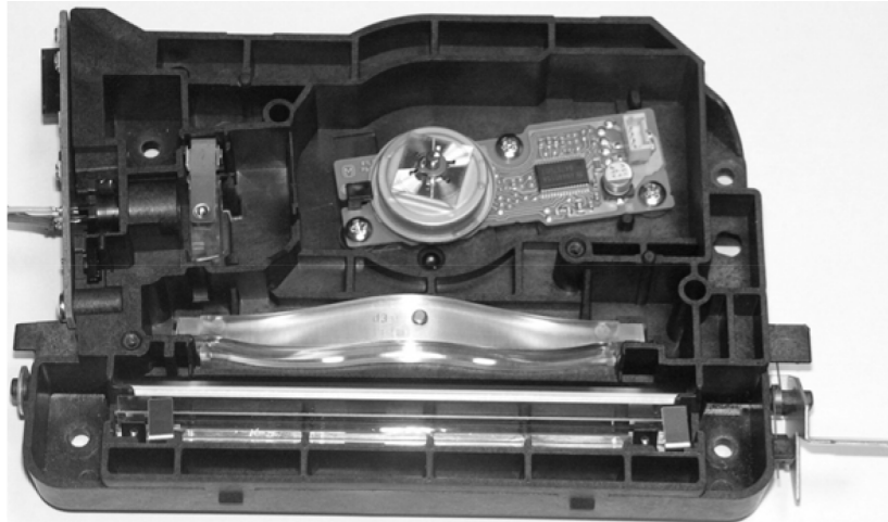
Figure 3. Example of a photoconductor exposure system used in standard laser printers (HP LaserJet P2035).
