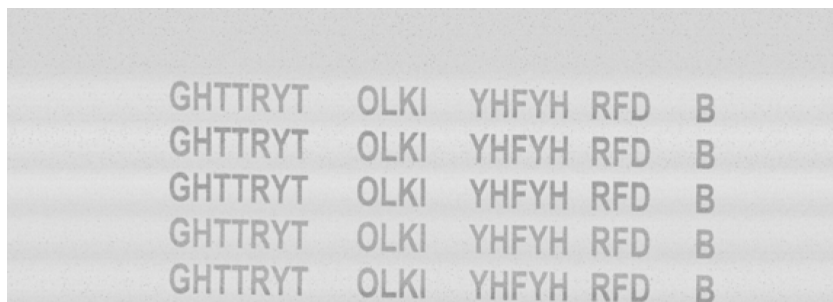
Figure 7. Fragment of a recreated image for revealing emission source in the form of a typical laser printer (image inversion, original character size of 26 points); reception frequency f_o = 145 MHz, BW = 10 MHz; sampling frequency f_s = 62.5 Ms/s.
