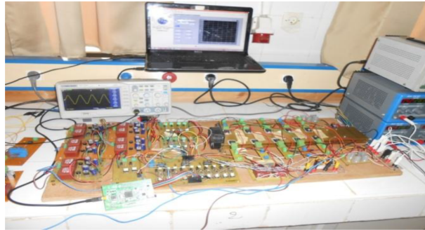
Figure 11. Laboratory prototype of the proposed inverter.
