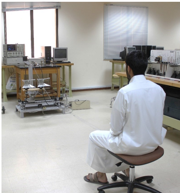
Figure 6. Picture of human being scanned at 3 m away from the antennas.
