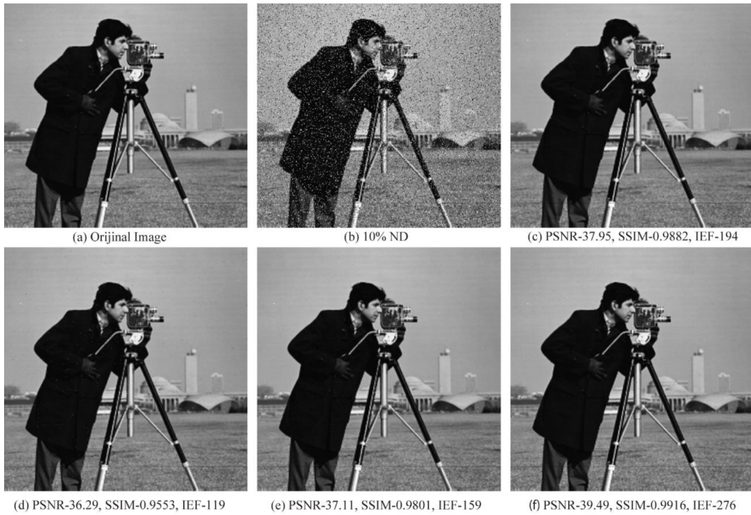
Figure 3. Cameraman image filter results: (a) original image, (b) image with 10% ND, (c) image after DBA, (d) image after MDBUTMF, (e) image after NAFSM, (h) image after BPDF.
